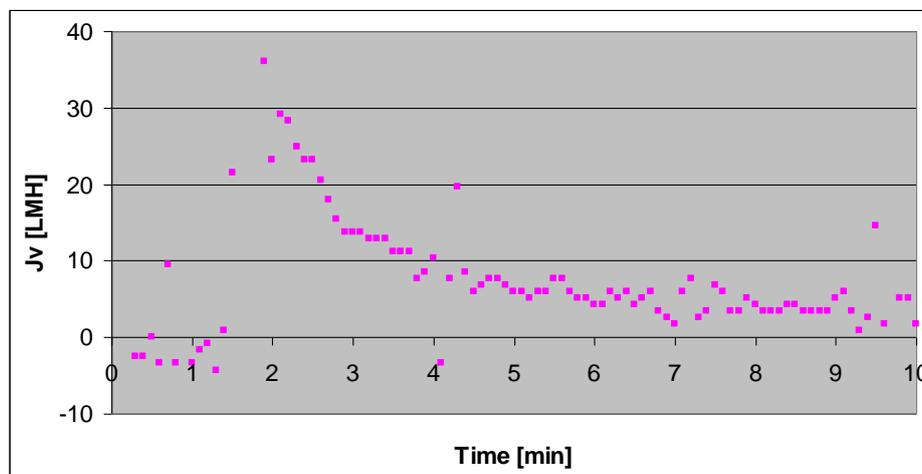
**Figure-5 – PRO Fluxes during first ten minutes.**
