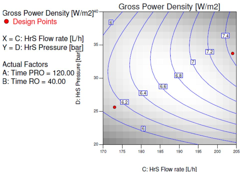
Figure 7 – Gross power density in PRO-RO process.
