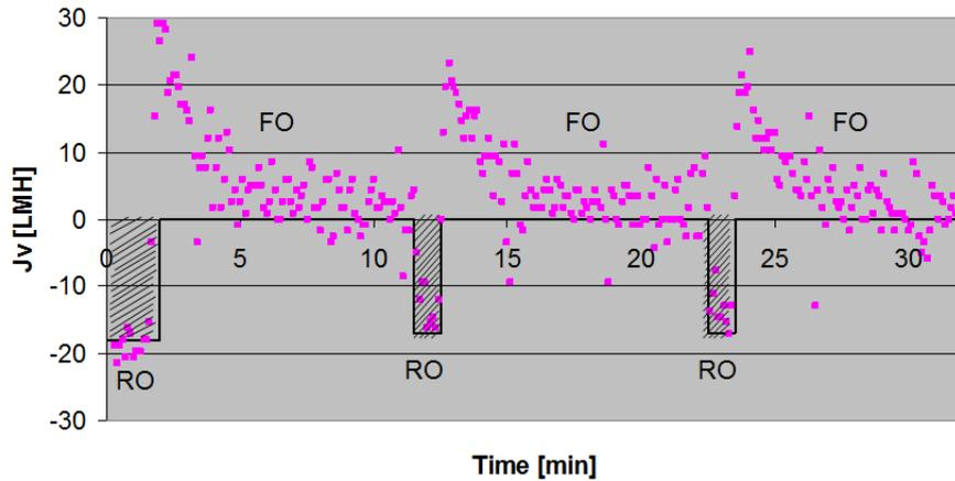
Figure 6 – Fluxes in PRO-RO process.
