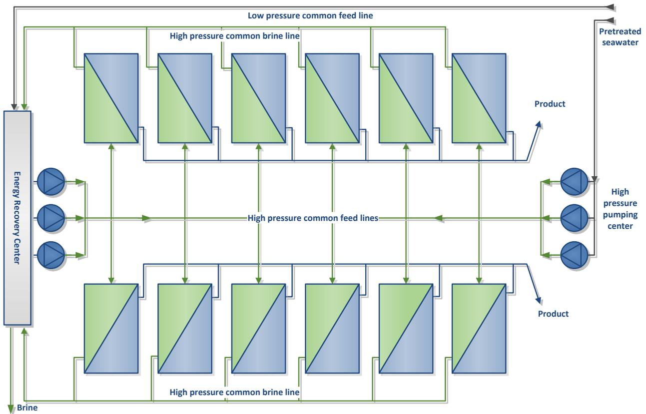
**Figure 5: IDE's Pressure Center Concept**
